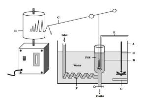
Isotonic Lever is used to record the contraction and load can not exceed 2 g
