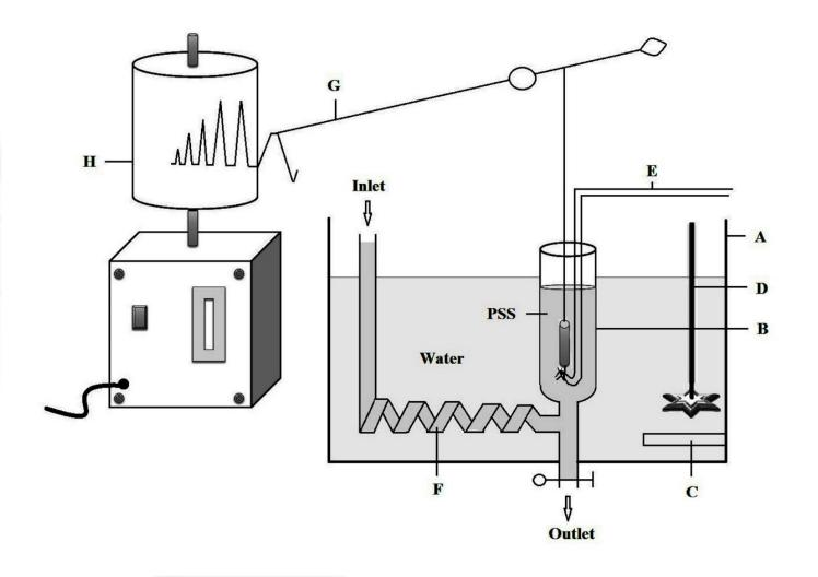
A: Water bath B: Organ Bath C: Thermostat D: Propeller E: Tissue holder tube F: Inlet coiled tube G: Liver H: Rotating drum
